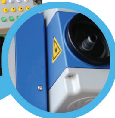
Laser technology (class 3 laser with a wavelength between 650 and 690 nm) for distance measurement
