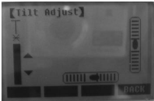
Fig.6 when the shadow is full, then the laser beam is Lightest.
